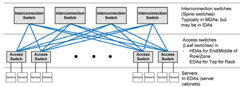
**LEGEND:** Active Switch-to-Switch Connection (solid blue line), Server connections (grey line), Category 8 Cabling / 25 or 40GBASE-T if channel length is under 30 meters (blue line), Category 8 Cabling / 25 or 40GBASE-T (grey line), Switch (grey box), Servers (white box), Repeated components (three dots)
