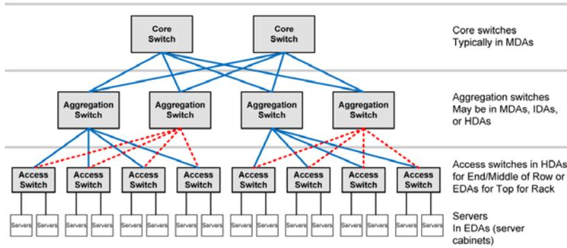
**LEGEND:** Active Switch-to-Switch Connection (solid blue line), Inactive Backup Switch-to-Switch Connection (dashed red line), Server connections (grey line), Category 8 Cabling / 25 or 40GBASE-T if channel length is under 30 meters (blue line), Category 8 Cabling / 25 or 40GBASE-T (grey line), Switch (grey box), Servers (white box)
