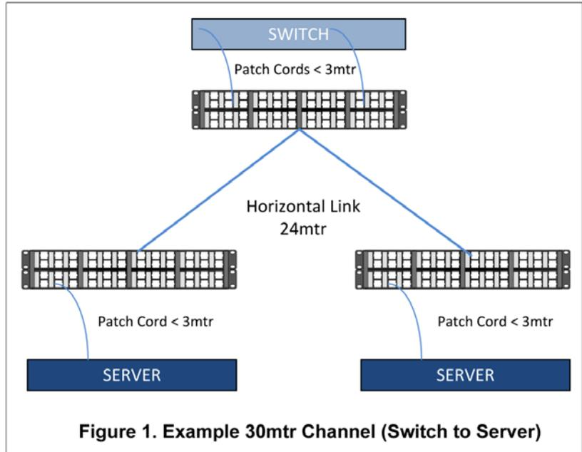
**Figure 1. Example 30mtr Channel (Switch to Server)**
